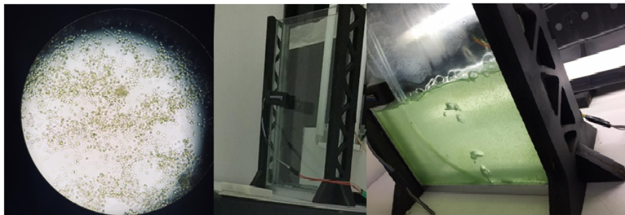
Fig. 4. Isolet Chlorella Vulgaris . and the photobioreactor used
